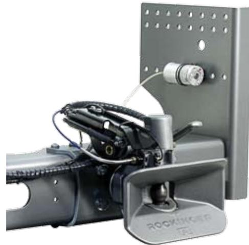
For ROCKINGER towing hitches too, LubeTronic AK can take over the time-consuming manual lubrication done during maintenance work. The cartridge, which is filled with special oil, is an ideal supplement to lubricating the coupling with grease. Thanks to its own battery, the LubeTronic AK requires no power supply from the vehicle, which also makes it ideally suited for retro-fitting. It has a useful life of up to 18 months and is available with one or two lubrication points.
